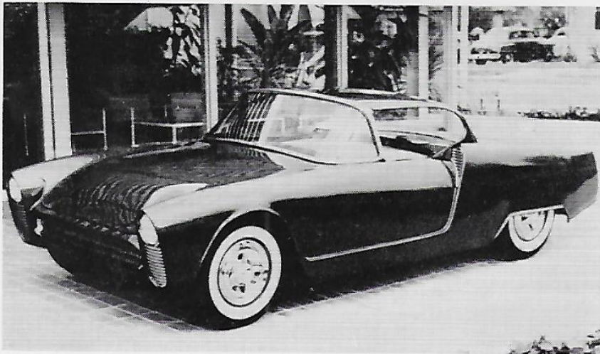
HENRY N. McCORMACK of Research designed and molded the fibreglas body of this beautiful sports car. The 2000-pound car, equipped with a '56 V-8 motor, packs approximately 425 horsepower.
